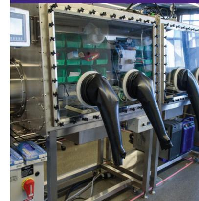
The Glovebox Inert Atmosphere (N<sub>2</sub>) Thin-film Fabrication and Testing core facility provides a range of equipment suitable for manufacturing and testing thin films of optically and electronically active materials inside a series of linked nitrogen-atmosphere gloveboxes. These materials are used in next-generation solar cells, LEDs, flexible and wearable electronic devices, and more, opening the doors to a brighter future in renewable energy science.
